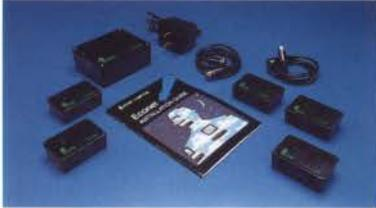
networks are joined together using Bridges. These provide high speed automatic connection between separate Econet networks ensuring areas of heavy network traffic are separated from each other to maximise network performance. One of the advantages of joining networks together in this way is that if one section of the network fails, the rest of the Econet system is not affected.
